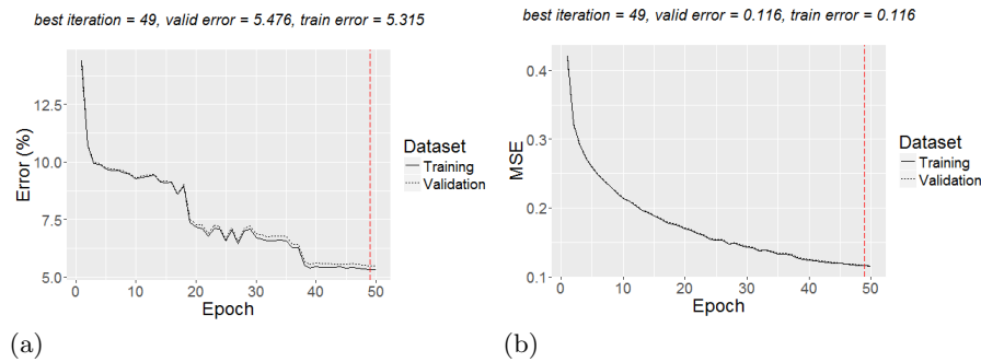
Fig. 7. Errors for iterations with 16 internal nodes: (a) Classification error; (b) MSE
